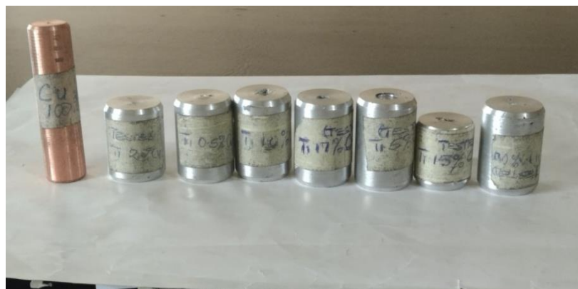
Fig 3: Developed beta phase Titanium copper specimens and copper specimen
